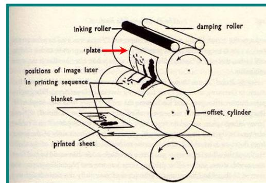
Figure 3.4 Offset printing process
