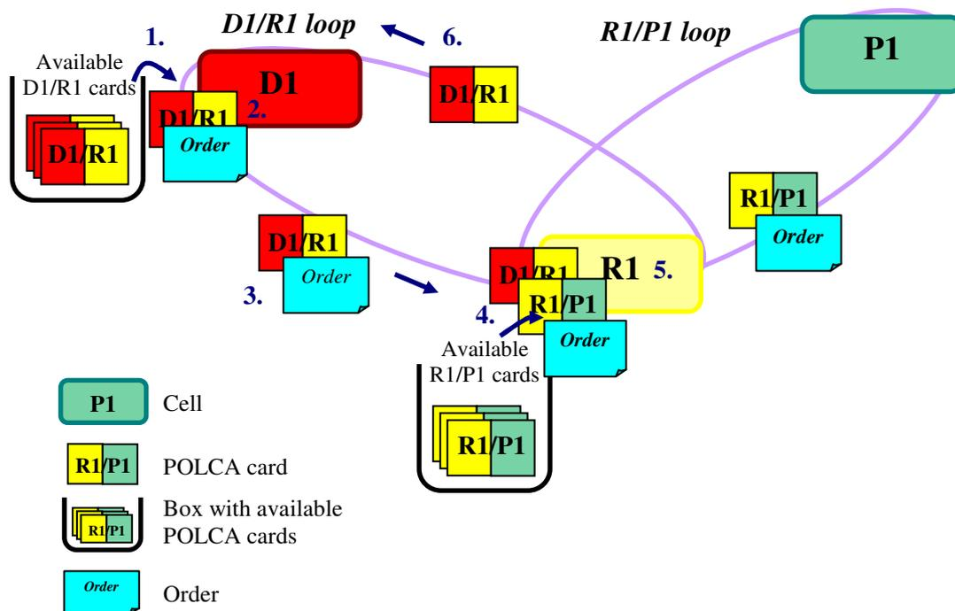
Figure 3.6 Loop that a POLCA card makes
